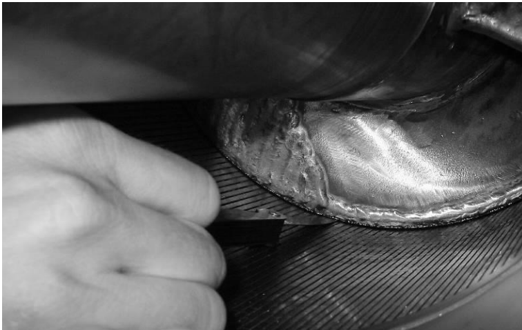
Fig. 13-17 Measuring of the working gap between the screen and the auger; the gap is measured on the bottom side of the screen while the machine is at rest. The measurement yields two times the working width because the screen rests on the top of the auger when the machine is not running.
