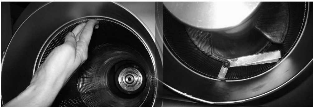
Fig. 13-13 Movable screen in the separator, inspection of the floating capacity by hand (left)
