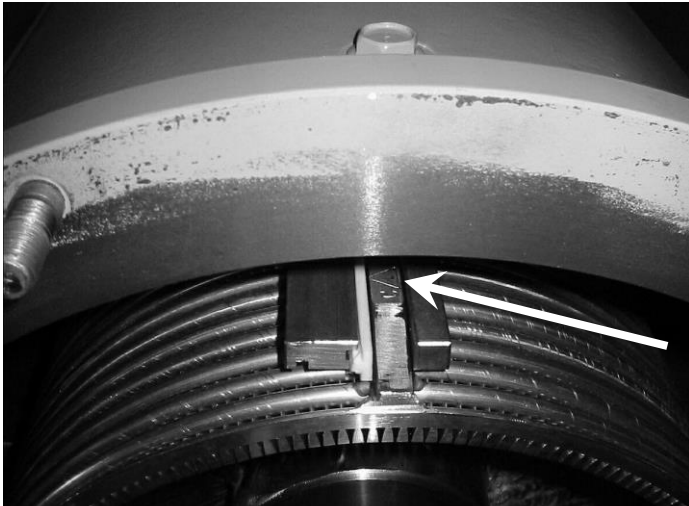
Fig. 13-12 Screen installation position, stamped triangle at top and toward the front of the separator
